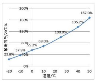
Sensor Zero Drift upon variable temperature
